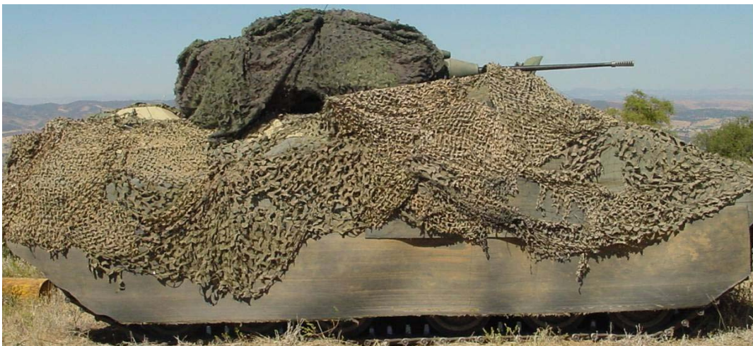
Figure 9a and 9b. M2A2 Bradley with depot level camouflage - conveyer belt over the vehicle surface augmented by a Colebrand (UK) Solar Blanket, and 2 types of US Camouflage Nets, the LCSS (Lightweight Camouflage Screen System) and ULCANS (Ultra Lightweight Camouflage Net System)
